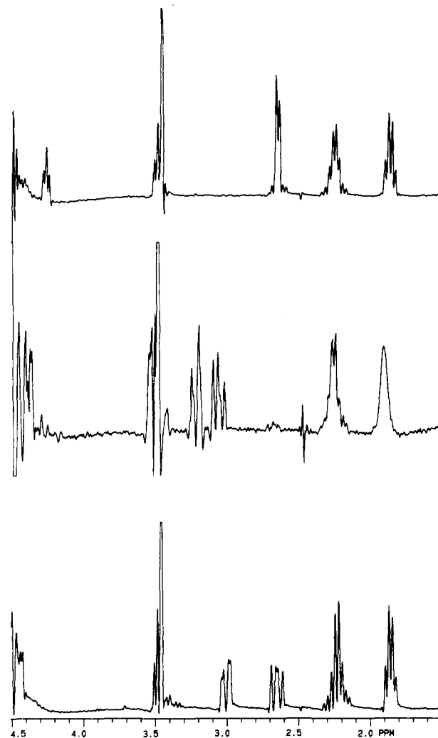
Figure 1. Proton NMR spectra of glutathione, the glutathione-chromium(VI)-thioester, and oxidized glutathione. (top) The 300-MHz 1 H NMR spectrum of 0.040 M GSH in D 2 O. The following conditions were used: pH* = 5.7, I = 1.5 M. The 256 transients were accumulated at 277 K. (middle) 1 H NMR spectrum of the reaction mixture of 0.040 M potassium dichromate and 0.040 M GSH in D 2 O. The following conditions were used: I = 1.5 M, pH* varied from 5.6 to 5.7. The 256 transients were accumulated with an acquisition time of 0.4 s and a delay between pulses of 1.0 s at 277 K. The spectrum was acquired from 11–17 min after mixing. (bottom) 1 H NMR spectrum of 0.020 M GSSG acquired under the same conditions as the top spectrum.
