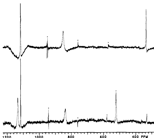
Figure 3. A comparison between the ^{17}\text{O} NMR spectra of chromium(VI) and the reaction mixture containing the \text{GSCrO}_3^- complex. (top) A 40.662-MHz ^{17}\text{O} NMR spectrum of 0.075 M potassium dichromate in 95% \text{H}_2\text{O}/5\% \text{D}_2\text{O} enriched \sim 10\% in ^{17}\text{O} . The following conditions were used: I = 1.5 M, \text{pH} = 5.2 . Approximately 15 000 transients were accumulated with an acquisition time of 0.04 s at 277 K. 90^\circ pulses were employed, and 10 Hz of line broadening was used. The sweep width was 100 000 Hz. (bottom) An ^{17}\text{O} NMR spectrum of the reaction mixture of 0.039 M potassium dichromate and 0.039 M GSH in 95% \text{H}_2\text{O}/5\% \text{D}_2\text{O} enriched \sim 10\% in ^{17}\text{O} . The following conditions were used: I = 1.5 M, and initial pH of both reactants was 4.9. Approximately 11 000 transients were accumulated with an acquisition time of 0.04 s at 277 K. 90^\circ pulses were employed, and 10 Hz of line broadening was used. The sweep width was 100 000 Hz. The spectrum was acquired 13–26 min after mixing, and the pH varied from 5.6 to 5.7 over this time period. The peaks marked with “*” are artifacts.
